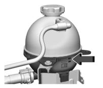
4. If the coolant level is not visible or needs to be adjusted within the reservoir, contact your dealer.
