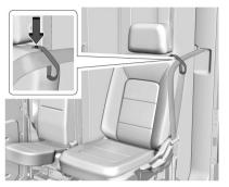
If the seat has a seat belt guide, the seat belt must be routed through the guide to properly position the shoulder belt. If the seat belt is not routed through the guide, slide the edge of the belt webbing through the opening on the guide. Be sure the belt is not twisted.
