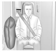
If equipped, the passenger side impact airbag is on the airbag trim cover adjacent to the jumpseat.
