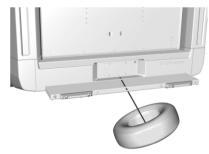
5. Tilt the tire toward the vehicle with some slack in the cable to access the tire/ wheel retainer.
