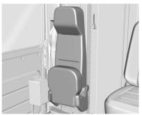
To use the jump seat, pull down on the seat cushion until the seat is in place. To store the seat, return the seat cushion to the upright position.
