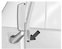
The remote key must be within 1 m (3 ft) of the door (including the sliding door) being opened or locked. Press the button near the door handle to open. See "Keyless Access Operation" in *Remote Key Operation*  $\Rightarrow$  7.
