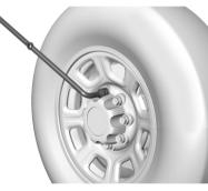
2. If the vehicle has a center cap with wheel nut caps, the wheel nut caps are designed to stay with the center cap after they are loosened. Remove the entire center cap.
