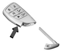
The mechanical key inside the remote key is used for the rear door.
