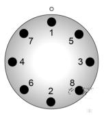
14. Tighten the nuts firmly in a crisscross sequence, as shown, by turning the wheel wrench clockwise.
