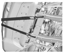
The vehicle has specific attachment points to be used to pull the vehicle onto a flatbed car carrier from a flat road surface. Do not use these attachment points to pull the vehicle from snow, mud, sand, or ditch.
