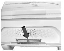
The vehicle may have a shutter system designed to help improve energy efficiency. Keep the shutter system clear of debris, snow and ice. If the check service vehicle soon light is activated, please check to see if the shutter system is clear of debris, snow or ice.
