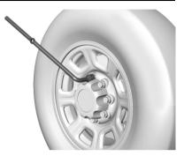
If the vehicle has a center cap with wheel nut caps, the wheel nut caps are designed to stay with the center cap after they are loosened. Remove the entire center cap.
