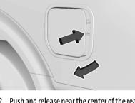
2. Push and release near the center of the rear edge of the charge port door to release the latch. Swing open the charge port door.
