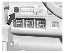
The Electric Parking Brake (EPB) can always be applied, even if the vehicle is off. In case of insufficient electrical power, the EPB cannot be applied or released. To prevent draining the battery, avoid unnecessary repeated cycles of the EPB.
