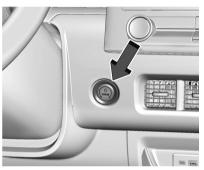
The vehicle has an electronic pushbutton start. The remote key must be in the vehicle for the system to operate. If the vehicle will not start, place the remote key in the transmitter pocket. See *Remote Key Operation*  $\Rightarrow$  7.
