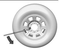
3. Use the wheel wrench and turn it counterclockwise to loosen the wheel nuts. Do not remove the wheel nuts yet.
