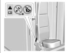
The label shown below is located on passenger side jump seat belt outboard anchor.
