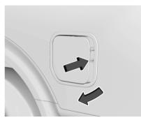
2. Push and release near the center of the rear edge of the charge port door to release the latch. Swing open the charge port door.
