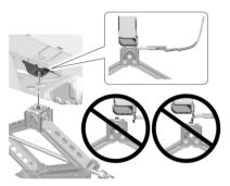
Ensure that the jack lift head is centered on the front or rear jacking pad. If equipped with a pin on the jack lift head, the pin must fit into the center of the hole in the jacking pad.
