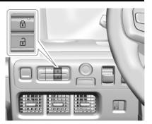
Press to lock all doors. The indicator light in the switch will illuminate when locked. See "Passive Locking" in *Remote Key Operation* ▷ 7.
